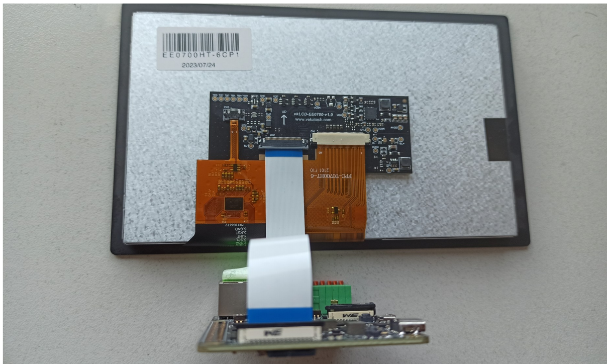
vkcz-dsi-vklcd-ee0700 display FPC cable orientation
